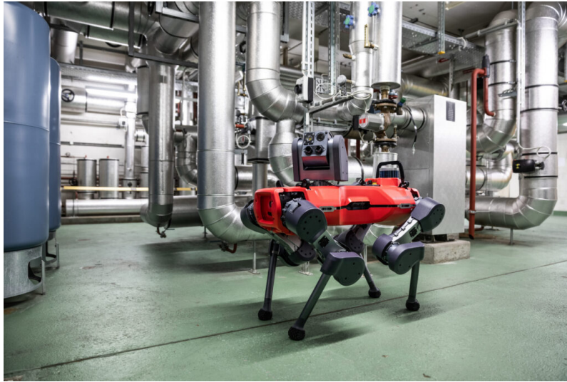
Figure 5.1. ANYmal performs inspection tasks in a typical, cluttered industrial environment. Reliable navigation is critical to its mission success and safety [7].
