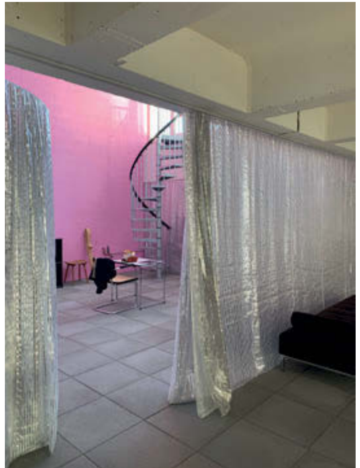
38 The insulation curtains—together with the adaptable green folding wall—permit the design of distinct thermal environments in an otherwise continuous indoor space.
