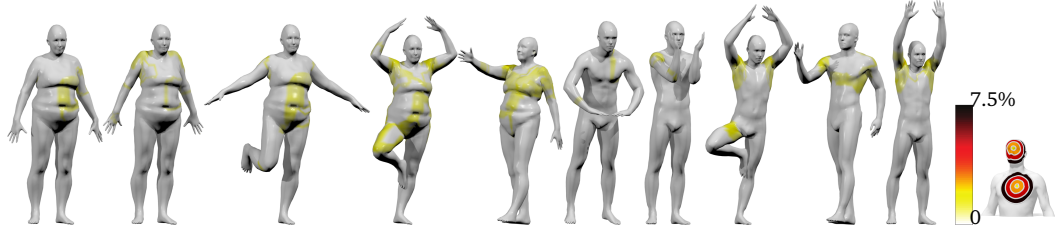
Figure 3.3. Pointwise error (geodesic distance from groundtruth) of MoNet on the FAUST humans dataset. For visualization clarity, the error values are saturated at 7.5% of the geodesic diameter, which corresponds to approximately 15 cm. Hot colors represent large errors.
