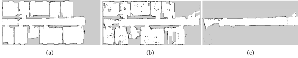
Figure 4.3. Different maps used in the experiments: (a) floor plan-like map, constructed by horizontally slicing a 3D point cloud captured with a FARO Focus X130 terrestrial laser scanner and (b) LiDAR-based occupancy grid map from GMapping [46] that was aligned to the FARO scan. (c) map built using GMapping, based on the recordings from the corridor scenario, which significantly deviates from the maps provided for localization.
