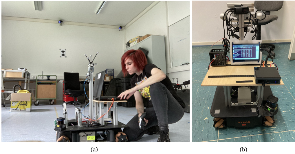
Figure 3.8. Transitioning from laptop dependency to onboard computation using an Intel NUC.
