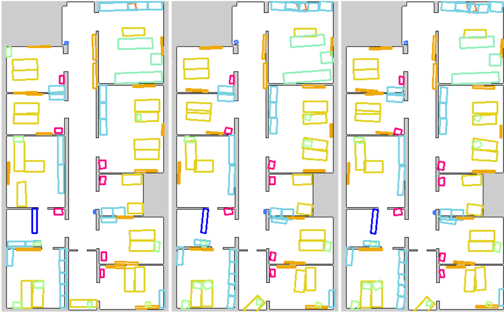
Figure 6.8. 2D projection for the 3 maps. Left: ground truth map obtained with terrestrial laser scanner. Middle: KP map. Right: map built using scan matching (ICP).
