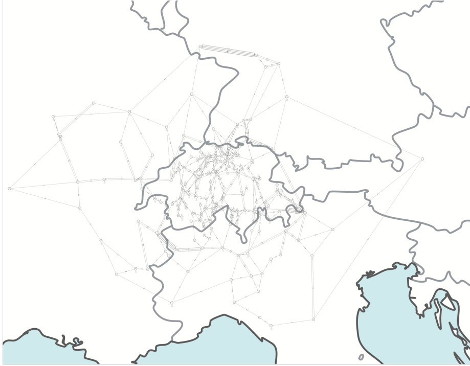
Figure 1.2: Topology of the Swiss grid with the external nodes in the neighboring countries.
