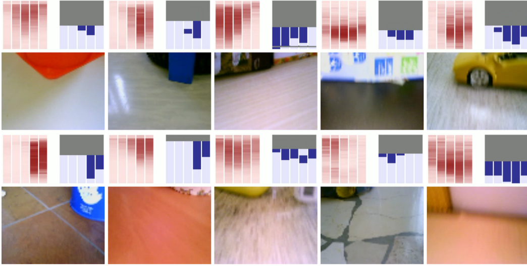
Figure 3.5. 10 instances from the acquired dataset, each coming from a different scenario (top row: scenarios 1 to 5; bottom row: 6 to 10). For each instance, we show the camera image (bottom) and the 31 \times 5 ground truth labels as a blue matrix (top right): one row per distance, one column per sensor; dark = obstacle detected; light = no obstacle detected; distances masked by gray rectangles correspond to unknown labels (due to the robot never reaching the corresponding pose). The red heatmap at the top left shows the predictions of a model trained on the other 9 scenarios.
