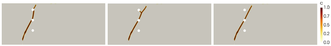
Fig. 8. Simulation results for asymmetrically notched beam test. Left: The solution obtained using the AM methods. Middle: The solution obtained using the ASPIN method. Right: The solution obtained using the MSPIN method.
