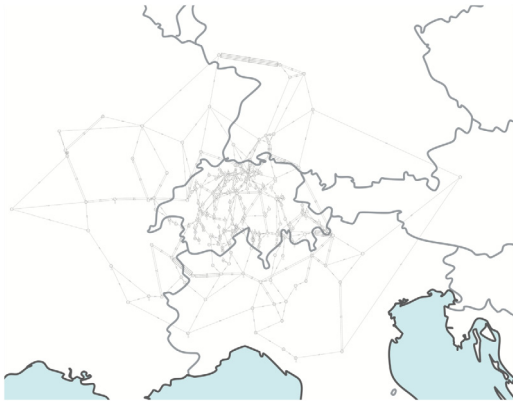
Fig. 2. Topology of the Swiss grid with the external nodes in the neighboring countries.
