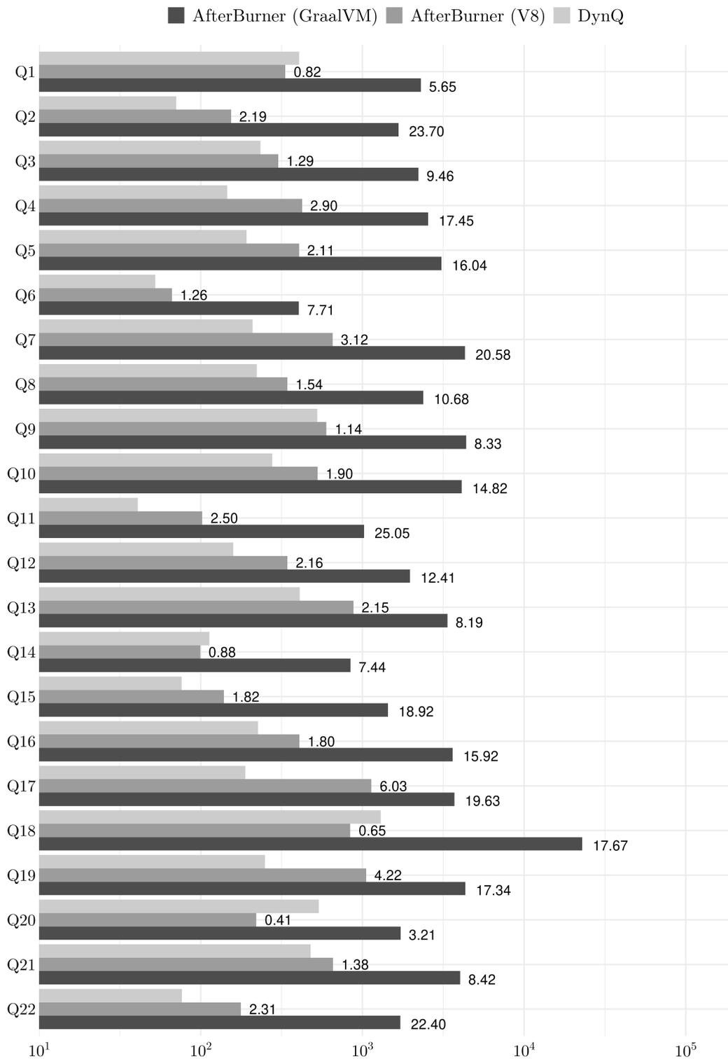
Figure 6.7. JS TPC-H benchmark on AfterBurner (SF-1).
