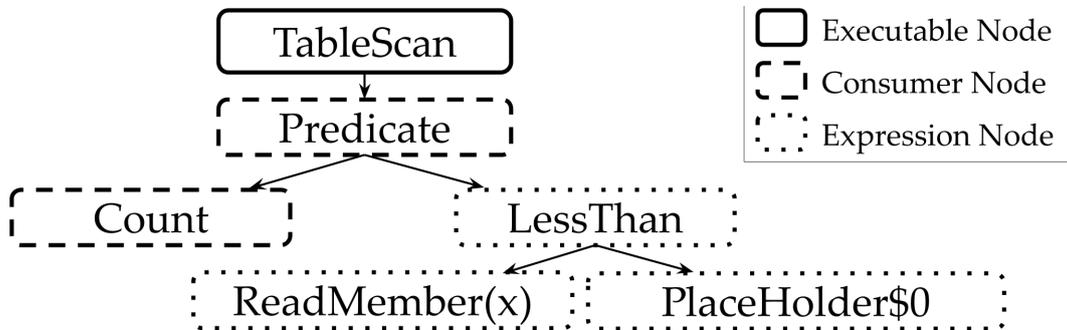
Figure 5.2. AST generated by DynQ for the prepared statement in Figure 5.1.
