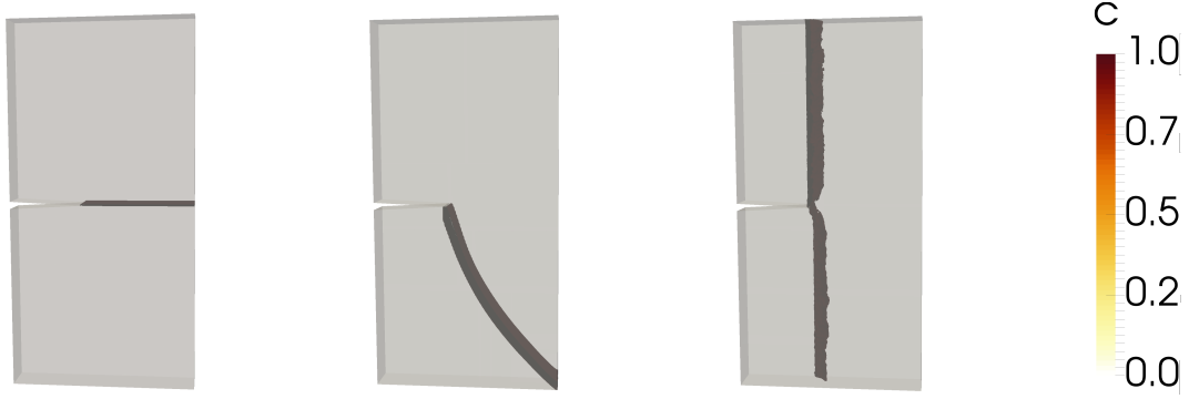
Figure 4.5: Iso-surfaces of the damage in the reference configuration for c = 0.99 for tension, shear, tear tests (from left to right). The presented results originate from an numerical experiment with approx. 105 thousand dofs.
