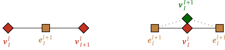
Figure A.3: Catmull–Clark boundary subdivision. Left : Edge midpoint construction (brown square). Right : Reposition of coarse-level point v_I^l (red diamond) into v_I^{l+1} (green diamond).
