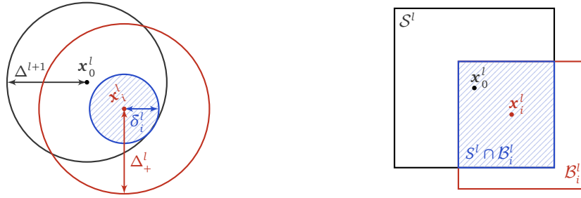
Figure 2.8: Preservation of the fine-level trust-region radius. Left: The trust-region radius defined by the \ell_2 -norm. Right: The trust-region radius defined by the \ell_\infty -norm.
