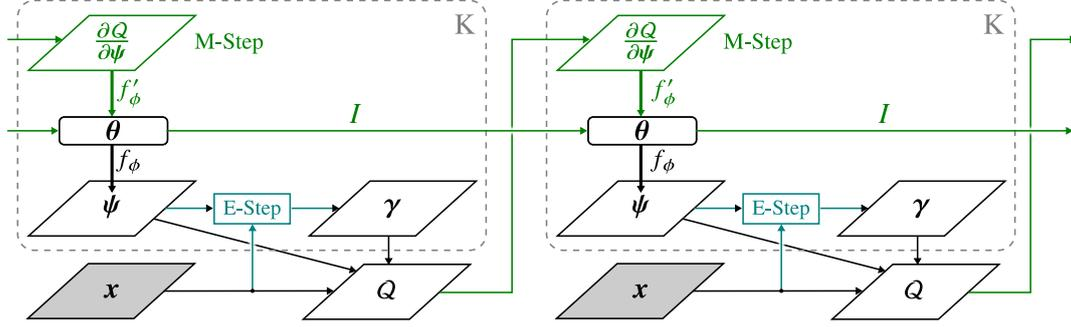
Figure 4.2. Illustration of the unrolled computational graph of generalized EM for the neural spatial mixture model under consideration. By backpropagating gradients through this graph (using backpropagation through time) it becomes possible to train the neural network parameters  $\phi$  based on an appropriate “outer” loss. Two steps of this trainable clustering procedure, which we call Neural Expectation Maximization (N-EM), are shown.
