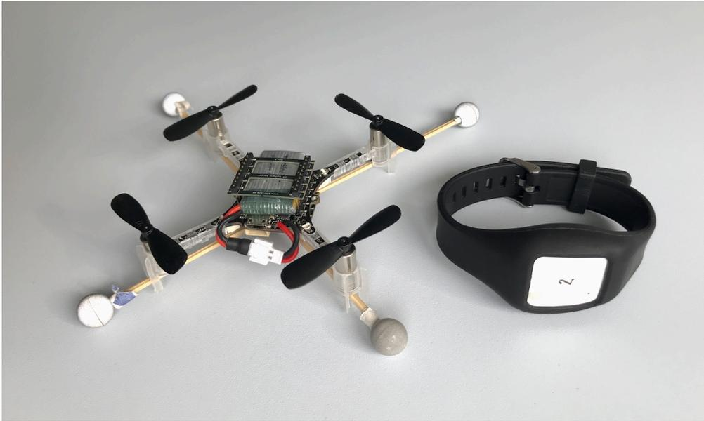
Figure 3.5. The hardware used in the experiments: (left) Bitcraze Crazyflie 2.0 quadrotor with retro-reflective markers for motion capture system; (right) Mbi-entlab MetaWearR+ IMU bracelet.
