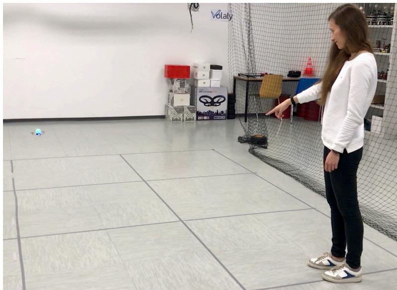
*Figure 1.1.* The user controls a miniature drone (Bitcraze Crazyflie 2.0) with pointing gestures acquired with a wearable IMU sensor (Mbientlab MetaMotionR+) placed on the user's wrist.
