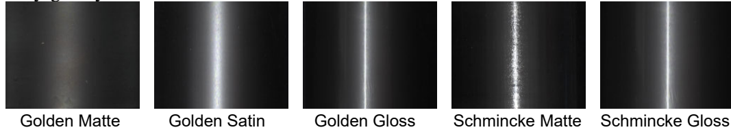
Figure 8.6. Photos of our printed varnishes on a cylindrical setup with a line light source.
