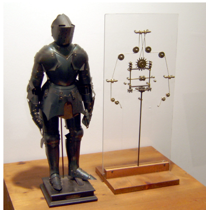
Figure 1.1. Mechanical Knight A humanoid designed by Leonardo da Vinci; the robot can move through a mechanical contraption connected to ‘tendons’.
