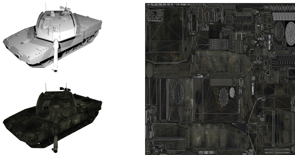
Figure 3.7. A 3D triangle mesh on the left top. Below is the same model with a texture. The UV-Mapping for the texturing is shown on the right overlaying the texture.
