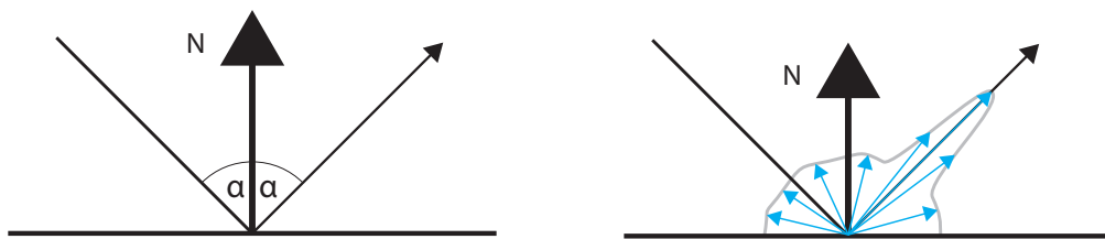
Figure 2.5. The incident angle is equal to the reflected angle for ideal specular reflection (left). For different materials the light flux is highest around the reflection vector and falls off quickly with increasing divergence from it (length of blue arrows on the right).
