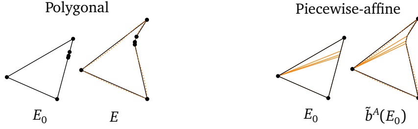
Figure 4.11. Comparison of b (orange dashed line) with its polygonal and piecewise-affine approximations (black solid line) for an element E_0 .
