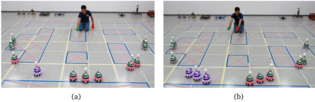
Figure 2.9. Spatial selection feedback from a robot swarm using colored LEDs. (a): Feedback from a spokes-robot robot. (b): Feedback from a group of robots.
