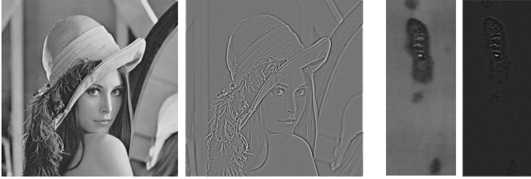
Figure 2.5. Examples of subtractive normalization on a conventional (left) and on a steel defect (right) image.
