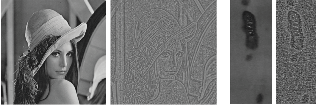
Figure 2.7. Examples of subtractive divisive normalization on a conventional (left) and on a steel defect (right) image.
