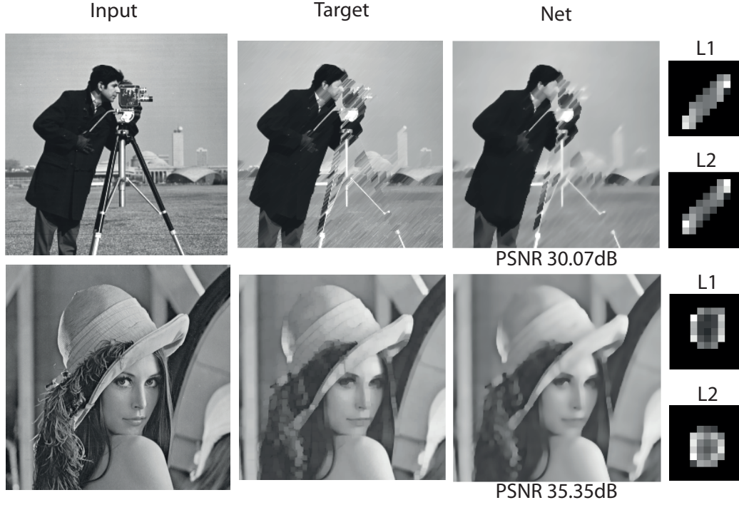
Figure 7.4. Top: an example of learning a closing operator where a line of length 10 and orientation 45^\circ is used. Bottom: opening with a square structuring element of size 5. The network closely matches the output and almost perfectly learns the structuring elements in both PConv layers.
