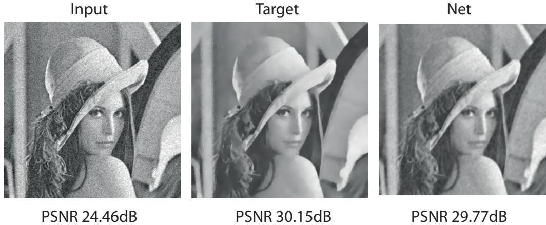
Figure 7.8. Total Variation (TV) task. The network has to learn to approximate the TV output (target) by means of averaging two filtering pipelines.
