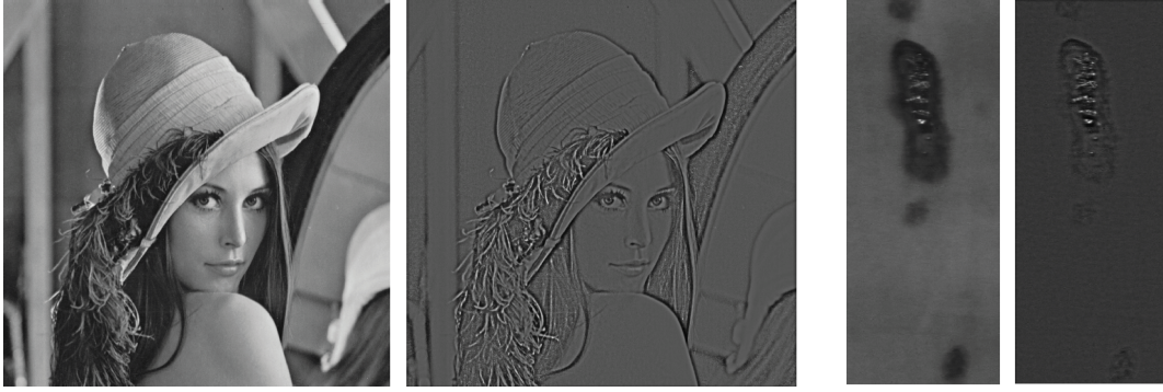
Figure 2.6. Examples of divisive normalization on a conventional (left) and on a steel defect (right) image.
