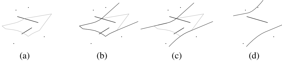
Figure A.2. Two line segments and (a) their order-2 Voronoi region; (b) the first opening of the boundary after removing two elements; (c) the disconnection of the boundary into two connected components; (d) removing one of the two segments does not reduce the number of connected components
