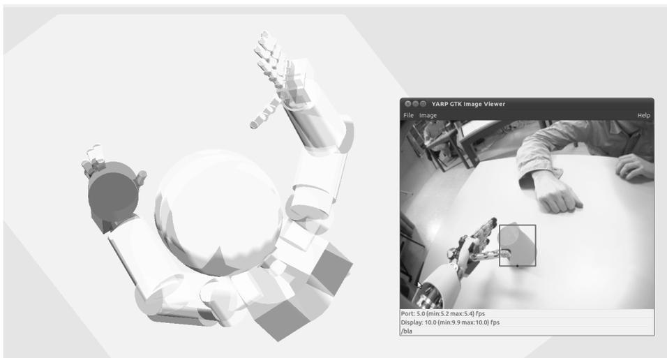
*Figure 3.37.* The object’s position is estimated and the world model of the *iCub* is updated. The evolved formula is used to calculate the position on the table based on the input images and the current encoder positions. *Note: The cup is placed directly under the arm, due to the parameters of the camera and the different perspective this is hard to see.*
