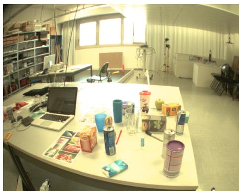
Figure 3.6. The distortion introduced by the system is clearly visible in this *iCub* camera image
