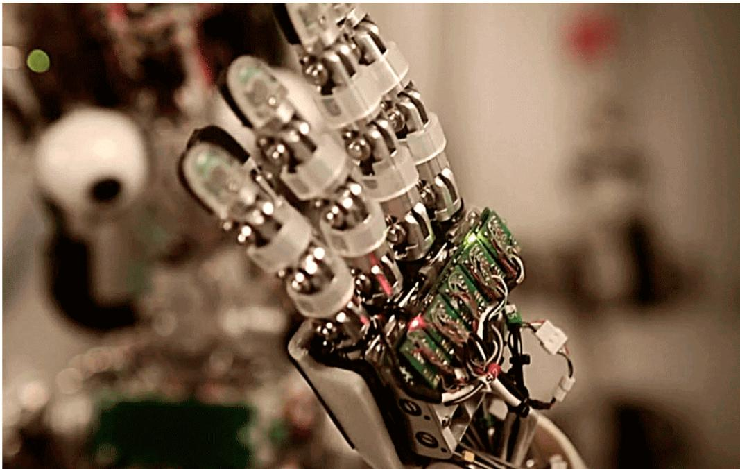
Figure 3.22. The *iCub*'s hands and fingers are quite complicated mechanically and complex to detect visually.
