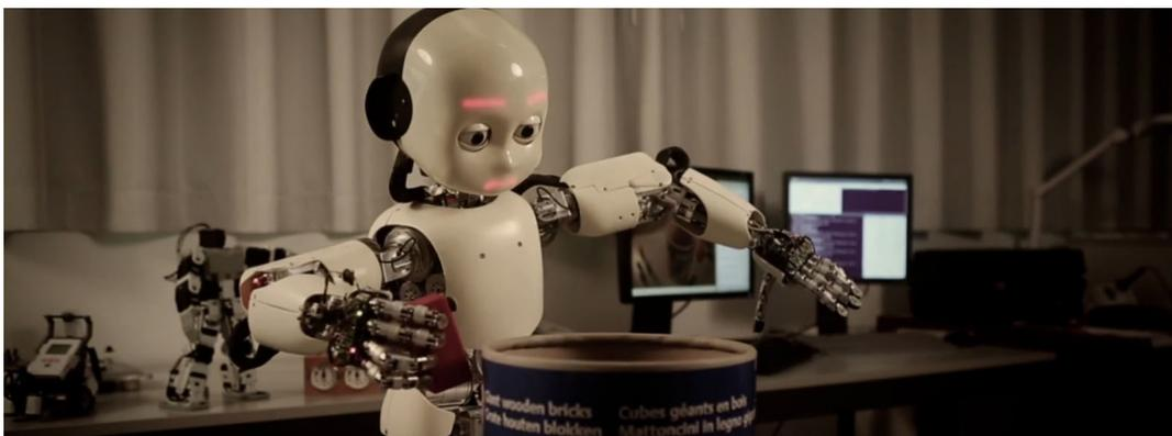
Figure 1.5. Our research platform, the *iCub* humanoid robot.
