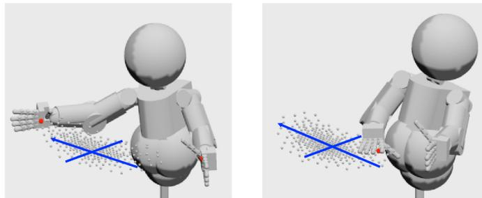
Figure 3.2. Hand marker positions (dots) for the task space: left/right, forward/back for the right hand, while the hand orientation is constrained in two different ways - Palm to the side (left). Palm down (right).
