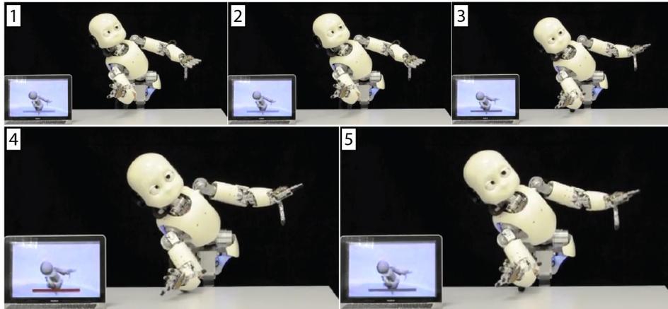
Figure 4.4. Time lapse images of MoBeE detecting impending collision with the table and invoking reflexive response. Collision is detected in frame 4, and response begins in frame 5.
