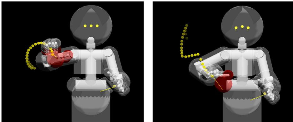
Figure A.1. These reaches were generated by the agent, which benefitted from intrinsically motivated exploration, after the learning experiments presented in section 8.4. The robot was put in a random state, a random reach target was selected (from the set of problems on which the agent has trained), and the RL system generated a policy. The yellow trails mark the history of hand poses throughout the execution of the policy.
