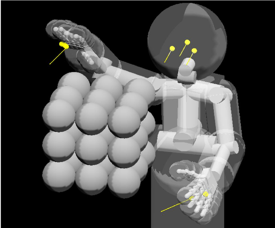
Figure 8.1. The set of 27 reach target objects (RL problems), arranged in a grid, which roughly covers the workspace of the iCub's right arm, without the aid of torso motion.
