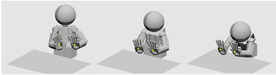
Figure 3.6. Push Forward - The height and relative position/orientation of the hands is constrained, and the 1D task space is to move them forward/back. The resulting map allows the robot to push a large object forward.
