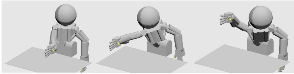
Figure 3.3. Raise a glass - The hand orientation is constrained, while the task space is the 3D workspace. The result is a map for pick-and-place with objects that must not be tipped over.
