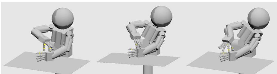
Figure 3.11. Unscrew - The position of both hands is constrained, as well as the orientation of the left hand and the palm normal direction of the right hand. The task space is the 1D orientation of the right hand about its palm normal. The resulting map would be suitable for unscrewing a bottle cap.
