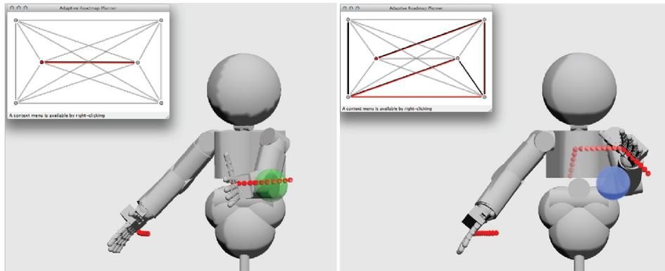
Figure 4.7. The iCub autonomously re-plans a motion to move from one side of the ball to the other. If the ball is not a solid object (top), the Agent moves the hand through it. When the ball is suddenly made an obstacle (bottom), the Agent quickly finds the path around it. The active plan is shown with red edges in the inset graphs.
