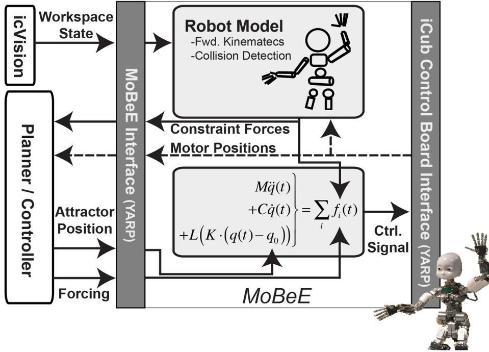
Figure 5.1. MoBeE 2.0 Simplified Architecture - The robot is controlled by a dynamical system (center-bottom, section 5.2), where  $q(t)$  is its configuration over time.  $M$ ,  $C$ , and  $K$ , are matrices containing mass, damping, and spring constants, respectively.  $q_0$  is an attractor, which can be set by the client program. Additionally, the client can force the dynamical system directly. Meanwhile, the robot model also forces the system to affect geometric and kinematic constraints.
