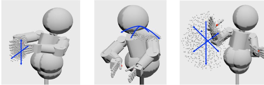
Figure 3.1. Marker positions (dots) for three different task spaces - Relative hand position/orientation is constrained, while the 2D task space is up/down, forward/back for the pair of hands (left). Absolute hand position/orientation is constrained, while the 2D task space is left/right, forward/back for the top of the torso (center). The elbow is constrained to stay down while the 3D task space is up/down, left/right, forward/back for the hand (right).
