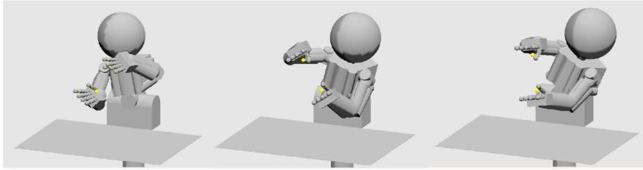
Figure 3.9. Bimanual Rotate - The relative positions and orientations of the hands are constrained, and the 1D task space is the angle of the palm normals (they are parallel with opposite orientation) in the up/down, left/right plane. The resulting map allows the robot to rotate a large object about the forward/back direction.
