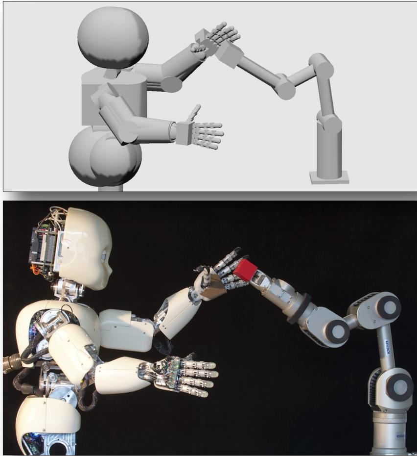
Figure 4.5. The iCub and Katana robots (bottom) cooperate in a shared workspace. Each robot is controlled via its own deliberate/reactive controller pair and the shared MoBeE framework (top).
