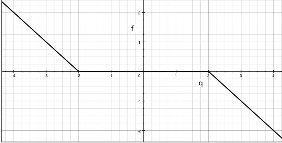
Figure 5.3. 1D Joint Limit Avoidance Function - Plot of equation 5.15 with joint limits,  $q_{min,i} = -3$  and  $q_{max,i} = 3$ , spring distance,  $\delta = 1$ , and maximum force,  $f_{max} = 1$  (at the joint limits).
