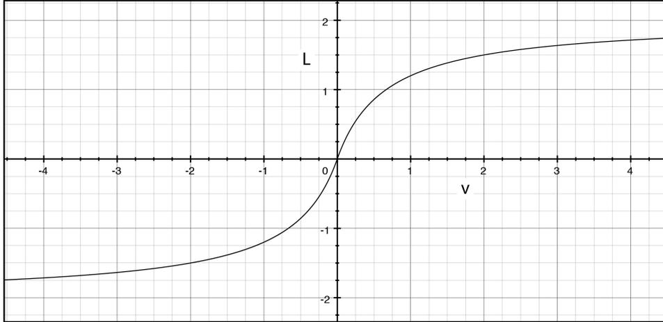
Figure 5.2. 1D Sigmoidal Lyapunov Function -  $L(v) = \frac{m \cdot v}{\frac{m}{k} + |v|}$ . Here, the maximum value is  $m = 2$ , and the maximum slope is  $k = 3$ .
