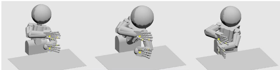
Figure 3.7. Push Over - The height and relative position/orientation of the hands is constrained, and the 1D task space is to move them left/right. The resulting map allows the robot to push a large object to the side.
