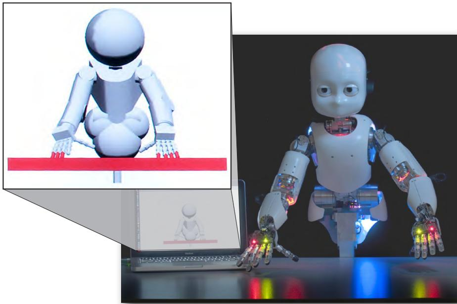
Figure 2.2. Impending Collision - The kinematic model detects impending collision between the iCub humanoid robot and a table. Darkened (red) geometries in the model (left) are colliding.
