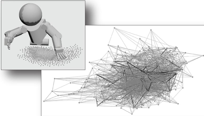
Figure 4.8. A large TRM is constructed by searching the configuration space for a set of approximately 5,000 ‘interesting’ poses. The scattered dots in the robot model (top-left) represent the position of the left hand as the robot assumes the pose associated with each vertex in the map (bottom-right).
