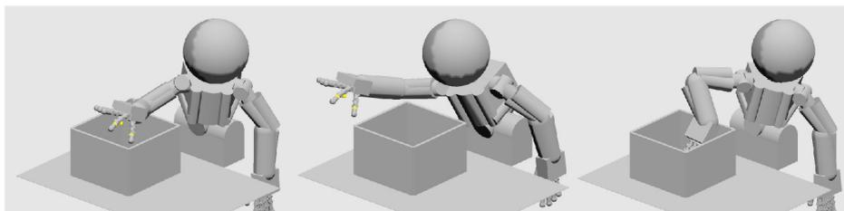
Figure 3.8. Reach Into - The robot is constrained not to collide with the box, and the task space is the 3D workspace for the hand. The resulting map allows the robot to pick/place from/into the box.
