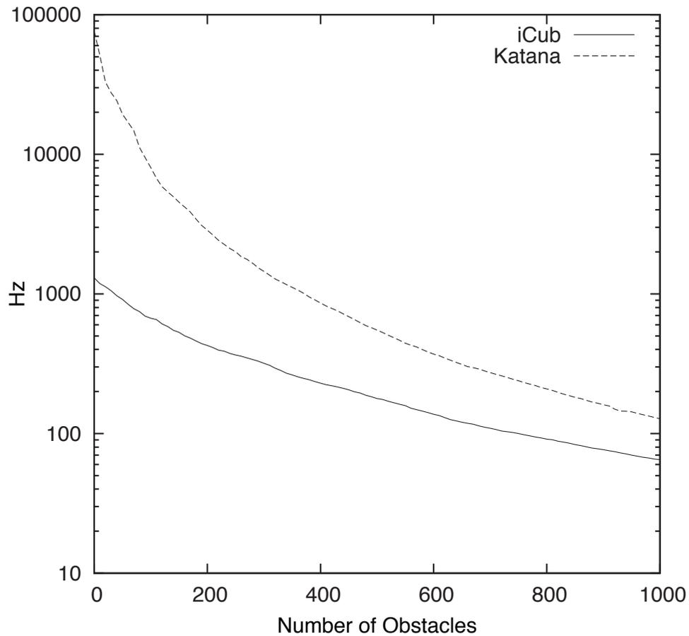
Figure 2.4. Kinematic Model Scalability - A simple robot model (Katana - 9 primitives) is compared with a complex one (iCub - 129 primitives). The curves show the number of times collision detection can be computed per second (y-axis) given a particular number of obstacles modeled in the robot's workspace (x-axis).
