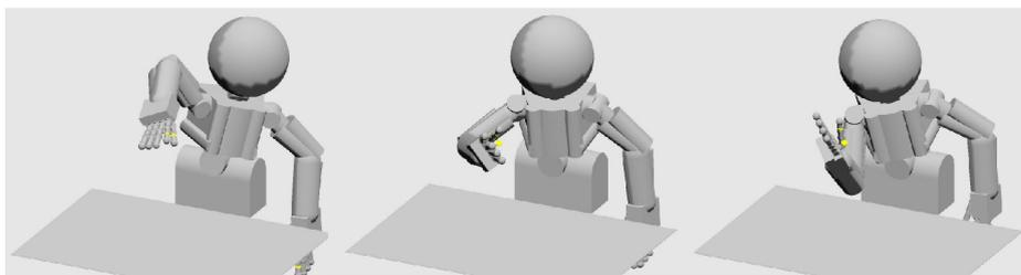
Figure 3.5. Inspect - the 3D position of the hand is constrained, and the task space is its angle with respect to the gaze direction. The resulting map rotates the hand (and any grasped object) in front of the eyes.
