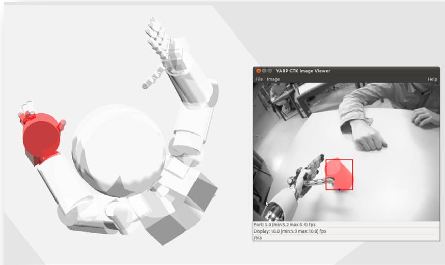
Figure 4.9. The resulting pose after reaching to the cup using an integrated Sensor, Agent, Controller system with the iCub robot. The inset (right) shows the iCub’s vision, overlaid with the (red) output of an Detector module. The cup, modeled as a cylinder, has been placed into the MoBeE model (left) by a Locator module. The roadmap used to plan the reach is pictured in figure 4.8.
