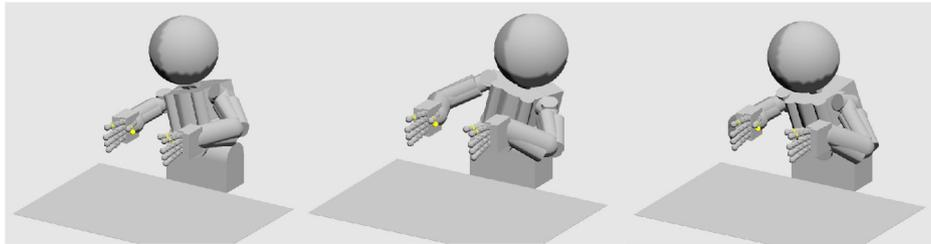
Figure 3.4. Bimanual Inspect - The position/orientation of both hands is constrained, while the task space moves the head around. This map is similar to figure 3.1 (center).
