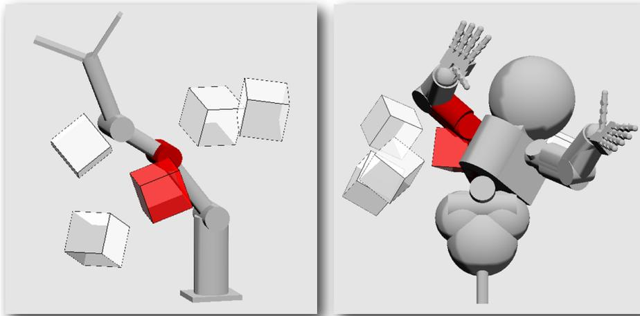
Figure 2.1. Kinematic Robot Models - The Katana arm (left) and the iCub humanoid (right) collide with random obstacles. Darkened (red) geometries are colliding.
