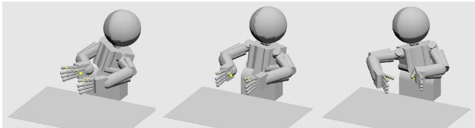
Figure 3.10. Bimanual Twist - The relative positions and orientations of the hands are constrained, and the 1D task space is the angle of the palm normals (they are parallel with opposite orientation) in the table plane. The resulting map allows the robot to rotate a large object about the up/down direction.
