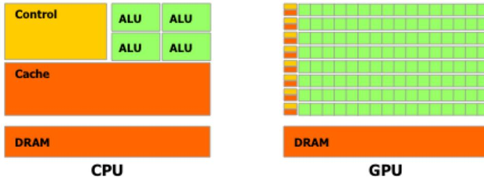
Figure 2.3. A typical CPU and GPU block scheme: the GPU devotes more transistors to data processing (from NVIDIA Corp. [2010b]).
